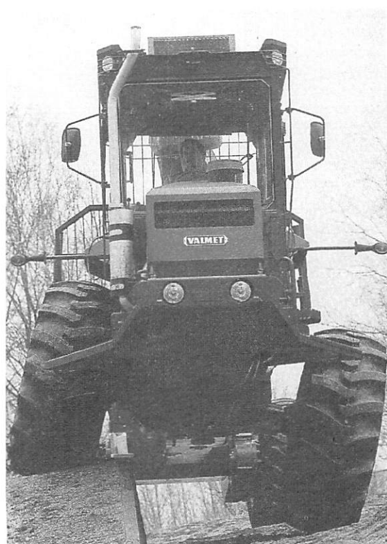
Fig 2. Valmet forwarder with swinging front axle.
