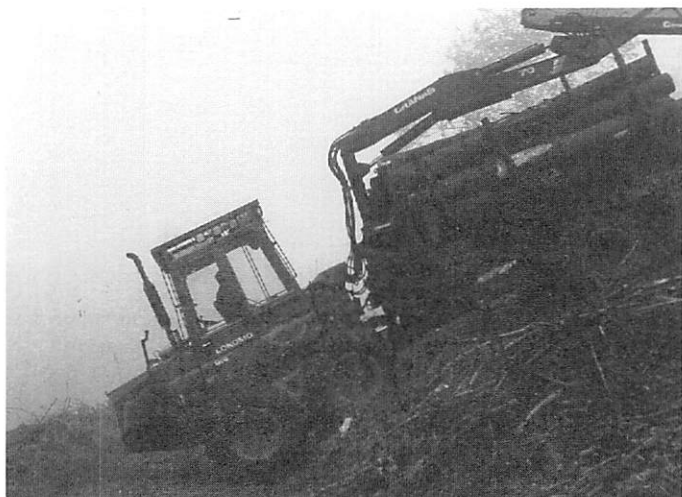
Fig 3. Forwarder descending a banking onto a forest road. Due to the steepness of the gradient the automatic difflock would be engaged making the sharp turn onto the roadline damaging to both machine and road. Great care is required to avoid overturning.
