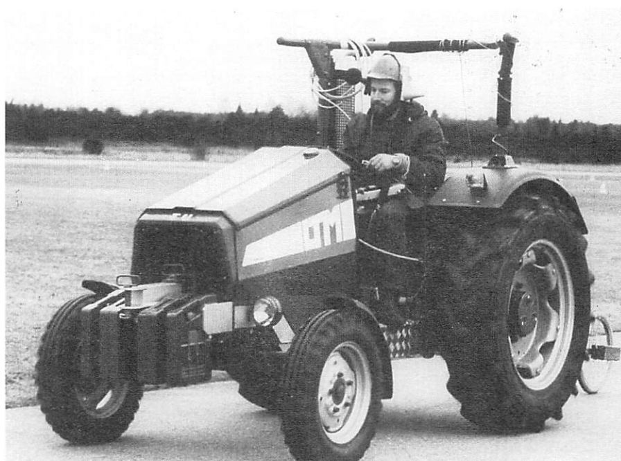
Fig 9. The Munich Research Tractor with infinitely variable steel belt transmission.
