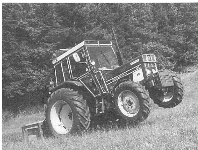
Fig 1. Examples of hazards on a slope: (left) tractor rearing when attempting to accelerate uphill, (right) trailer tipping sideways as a result of slope, speed and ground roughness.
