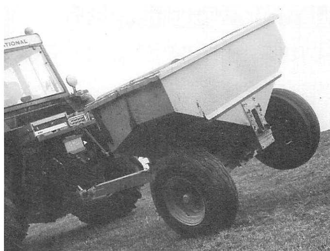
Fig 1. Examples of hazards on a slope: (left) tractor rearing when attempting to accelerate uphill, (right) trailer tipping sideways as a result of slope, speed and ground roughness.
