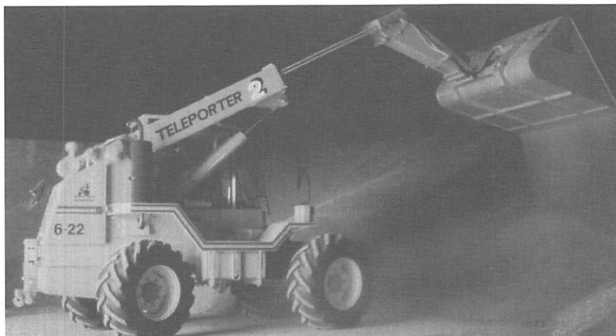
Fig 3. Workers can be isolated from dust by the use of cabs equipped with suitable air filtration systems.
