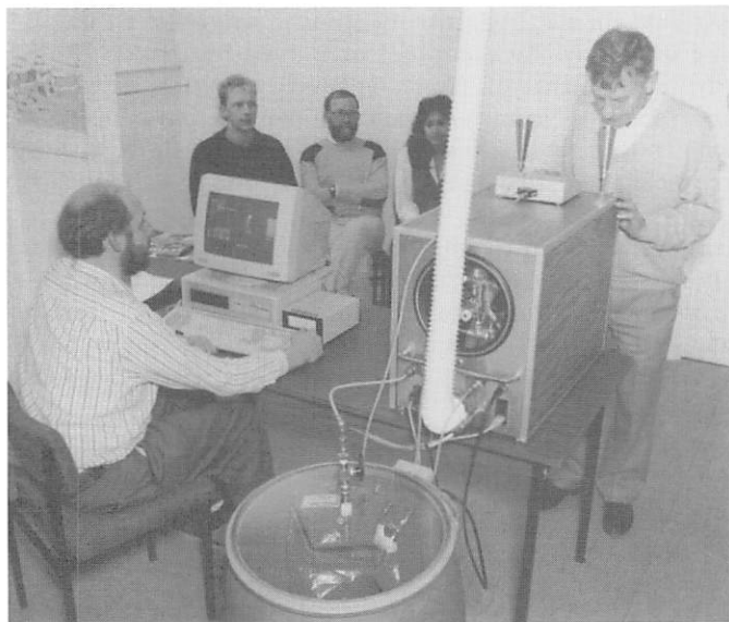
Offactometers in action, using members of the public to assess colour concentration, intensity, and offensiveness. The system is fully computer controlled, and uses samples collected in special bags.
