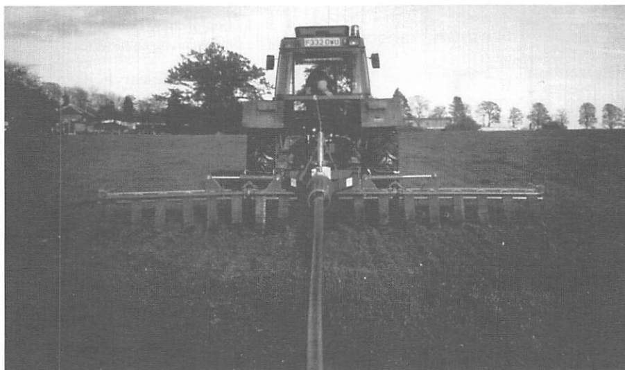
Fig 1. Drop pipe applicator connected to the umbilical drag hose and drawn by two wheel drive tractor.
