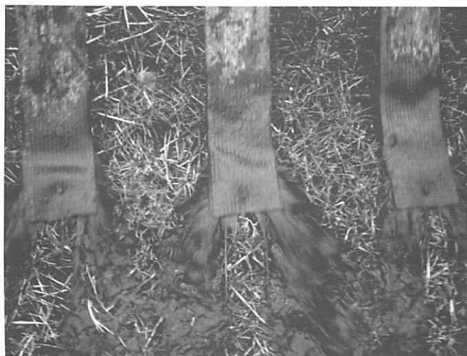
Fig 2. Distribution of slurry from drop pipes is directly onto the ground at low pressure with no atomisation.
