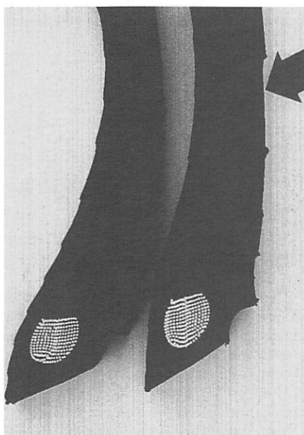
Fig 1. Section of forestry tyres showing extra thick side wall to give added protection on rough stony ground.
