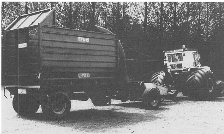
Fig 2. Reduced ground pressure forage harvesting equipment.
