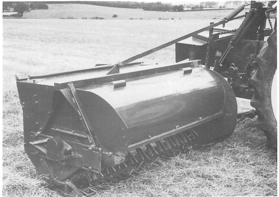
Fig 1. Early experimental field rig for evaluating a high-speed conditioning rotor with V-shaped steel spokes above a reciprocating cutterbar (Photo: Silsoe Research Institute).
