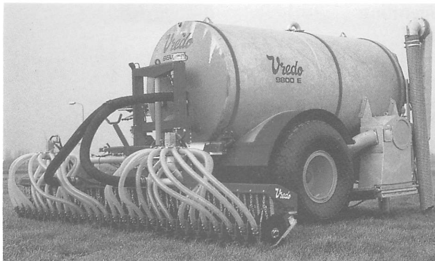
The Vredo range of advanced slurry injection equipment from Holland is now being handled by Horsch UK Limited. The equipment is based around a unique double disc injection unit which accurately places the slurry at 2"-3" depth with row spacings of 8". This system is suitable for injecting waste into grassland at rates of up to 35m 3 /ha.
