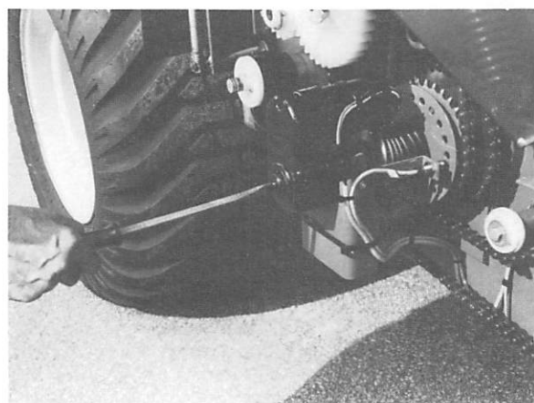
The electronic controlled Variator on a Tive 2206 drill jet.
