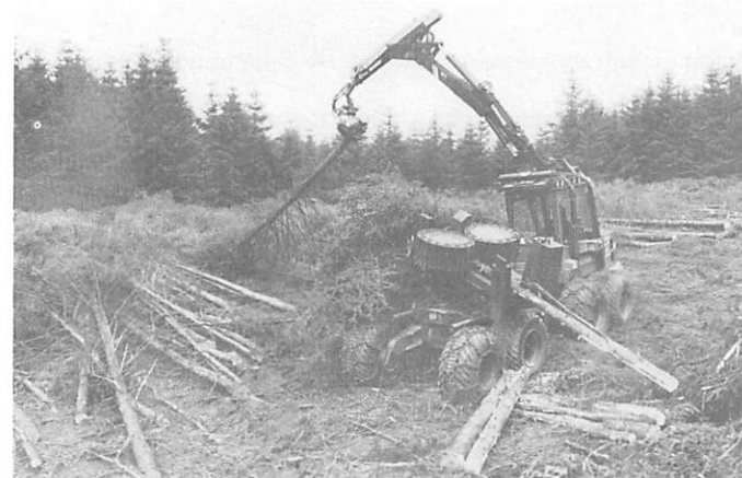
A Bruunett processor 678P. The machine is seen with one tree length being snedded and crosscut and one tree length being lifted by the grapple arm from the waiting row. Photo: Forestry Commission, Edinburgh.
