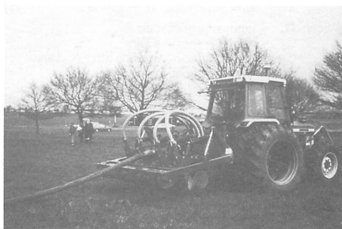
Fig 2. Umbilical injection system.
