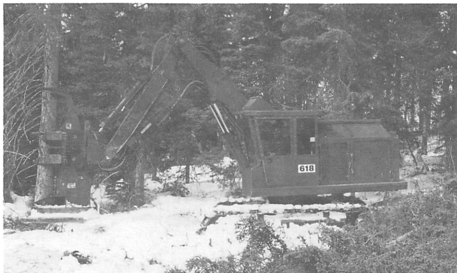
FMG Feller Buncher – holding only one tree but can take more.
