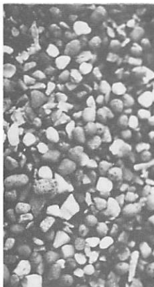
Rounded particles and angular rubber particles. High shock absorbency, not fluid.
