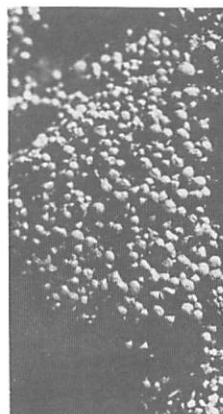
Rounded particles with high shock absorbency and ideal for a fluid system.
