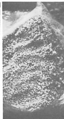
Angular sand particles. High critical tensions and only fluid in very dry conditions.
