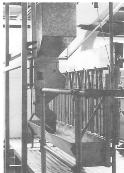
Fig 2. The tracked feed dispenser unit to allow individual feeding of experimental animals in the milking parlour.
