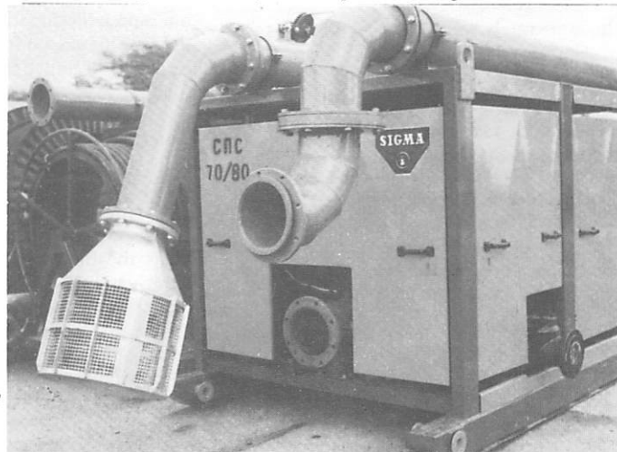
Seasonal translatable pumping station.
