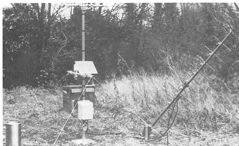
One of the budget weather stations manufactured by the Didcot Instrument Company for use in Botswana. The data collection platform is on the right.
