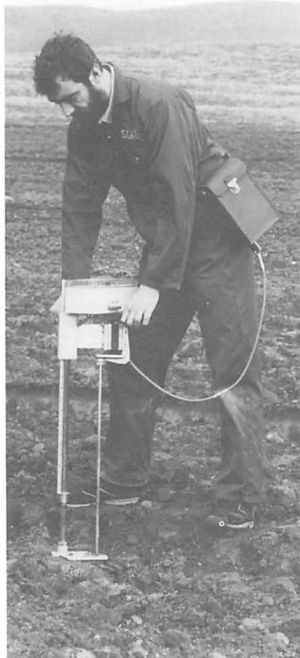
Bush recording soil penetrometer and associated data collector — designed by scientists in the Soil Engineering Dept of SCAE and produced commercially by Findlay, Irvine Ltd, Bog Road, Penicuik, Midlothian
