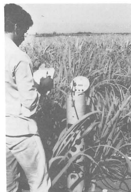
The Wallingford neutron probe soil moisture meter, developed at the Institute of Hydrology, being used on drip irrigation trials in Mauritius (photo: Institute of Hydrology)
