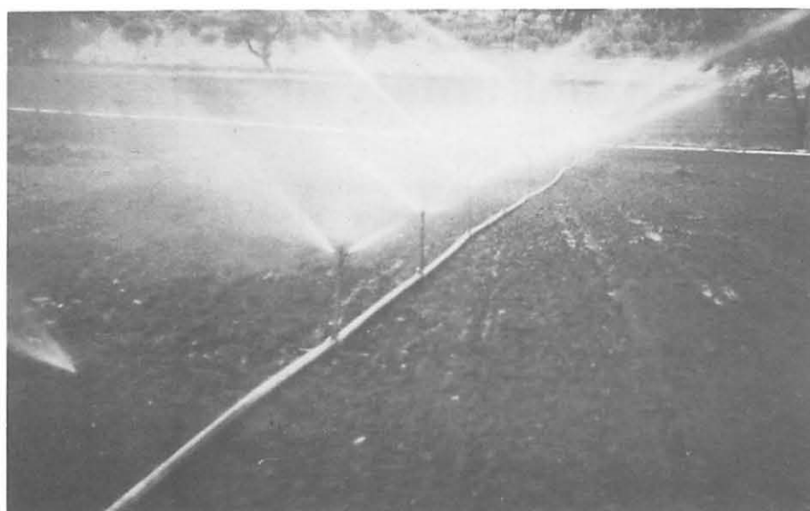
A rotary sprinkler irrigation system giving a near-uniform distribution pattern (photo: Wright Rain Ltd)
