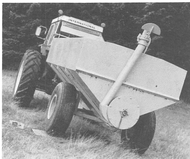
Fig 7. Accuracy experiment for the weighpad method on a preset slope provided by the tilt table.
