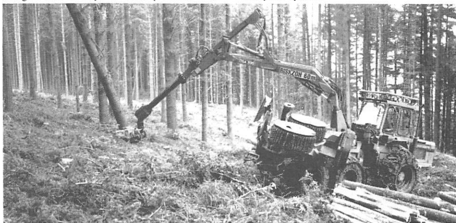
An OSA harvester felling a P38 Douglas fir. Kintyre Forest District, April 1987.
