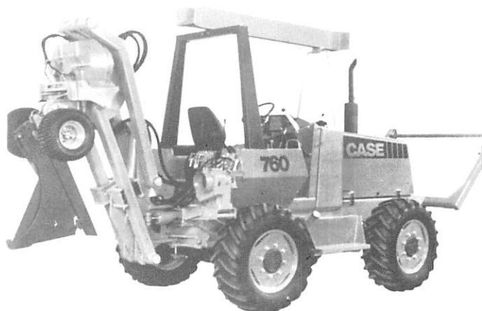
The new 760 Case trencher with 763 vibratory mole plough attachment supplied by L D Bourgein (Oxford) Ltd. (0865) 735420
