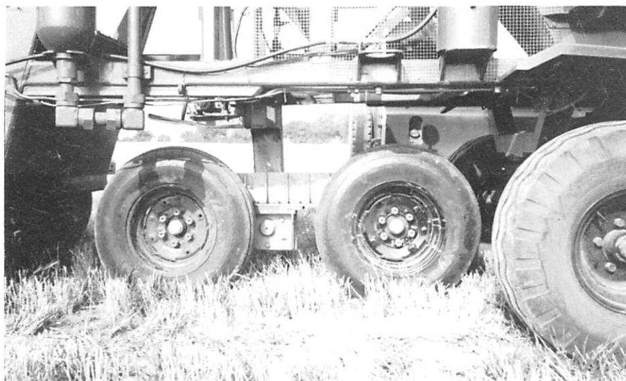
Fig 2. Tandem axle fitted to test rig.
