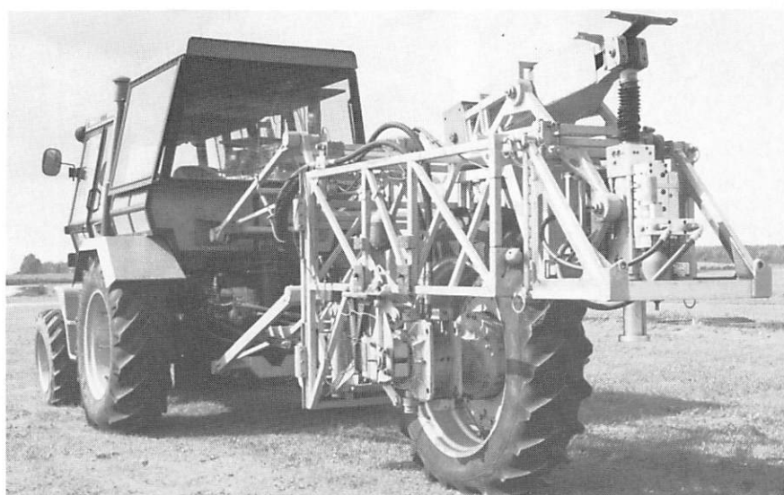
Fig 2 Single wheel tester used on tyre research (AFRC Engineering 'photo)
