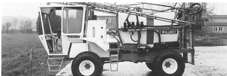
Fig 2 The Willmot Light spray 1548HY, a low ground pressure spraying rig which allows the application of pesticides throughout the year with minimal crop and soil damage
