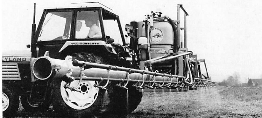
Fig 1 The Airtec Sprayer from Cleanacres Machinery incorporates both a liquid and an airfeed, giving a fully adjustable droplet spectrum
