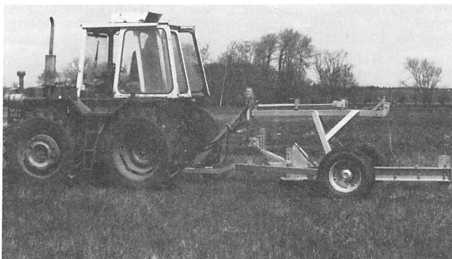
Fig 2 Floating beam mole plough designed at Silsoe College
