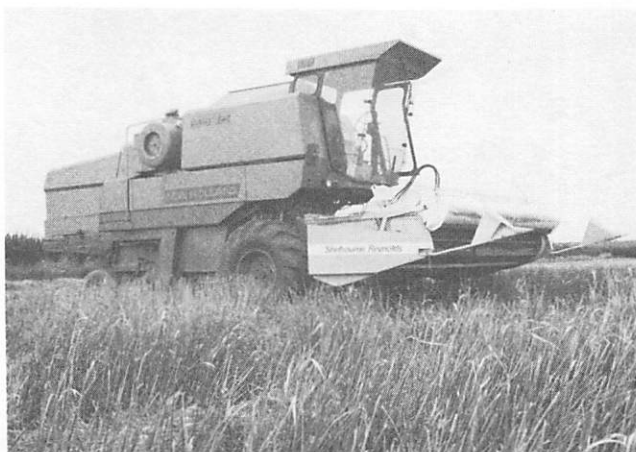
Fig 9 Commercial prototype stripper header built by Shelbourne Reynolds Engineering Ltd, Stanton, Nr Bury St Edmunds, Suffolk
