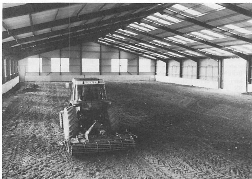
Fig 1 A power harrow under test in the Harper Adams Agricultural College covered soil working area
