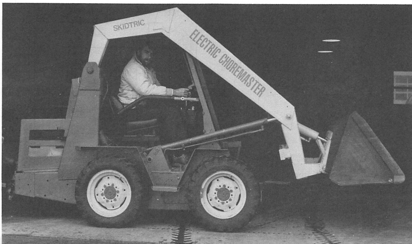
Fig 1 Battery powered skid-steertractor, driven by the author
