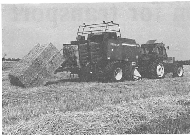
Fig 1 The Hesston 4800 baler makes a 500 kg straw bale
