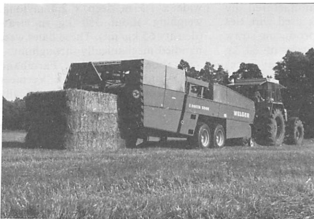
Fig 3 Three bales are accumulated within the Weger Delta 5000 baler
