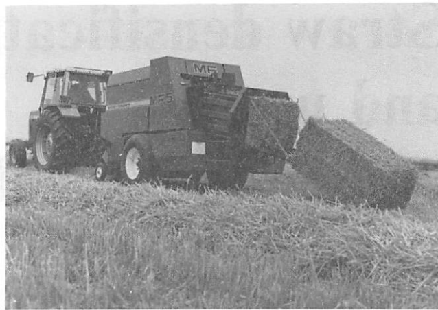
Fig 2 This Massey Ferguson MF5 baler produces a bale 800 mm square in cross section
