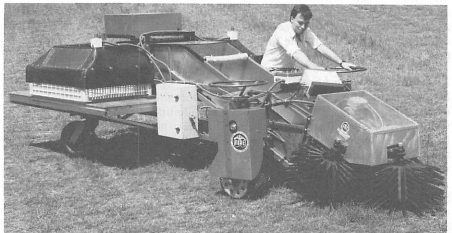
Fig 4 The NIAE broiler collecting machine designed to reduce injury to the birds (source NIAE)
