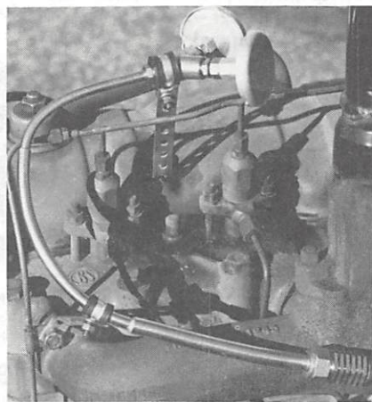
Fig 1 The 'Gefarator' exhaust aspirator fitted on the David Brown 996 tractor
