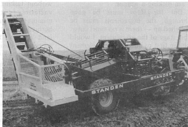
Fig 8 sugar beet cleaner – a NIAE improvement to an existing machine from an established company
