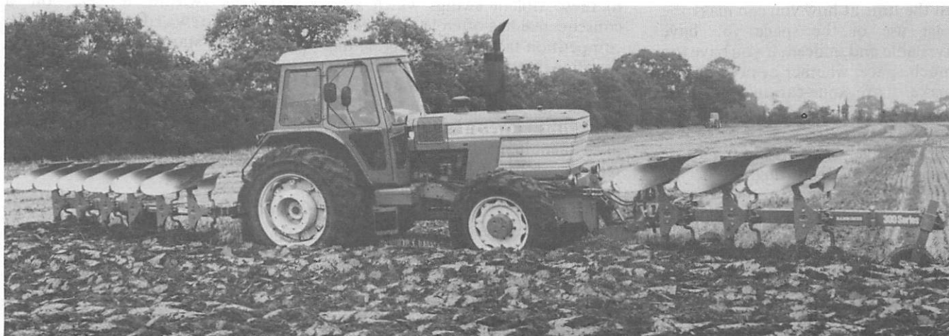
Fig 1 This 9-furrow "push-pull" ploughing combination incorporates the recently introduced TSR 300HD 6-furrow plough. It is operating on a medium heavy land farm in Suffolk, ploughing 35 cm wide furrows 23 cm deep with a 120 kW tractor (photograph: Ransomes Sims & Jefferies plc)
