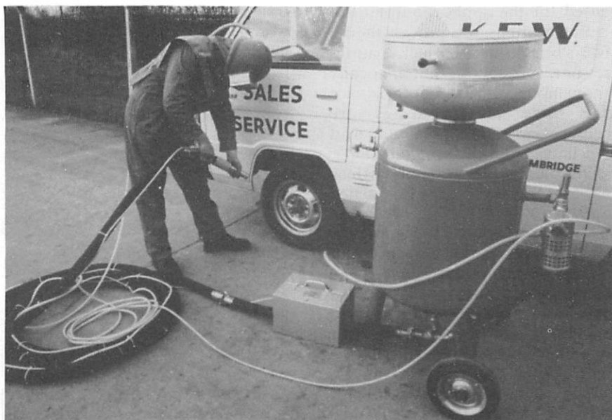
Fig 8 Portable, self-contained, gritblasting unit for preparatory treatment of metal surfaces
