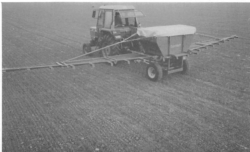
Fig 2 A trailed 12 metre pneumatic fertiliser spreader [AC Bamlett Ltd photograph]
