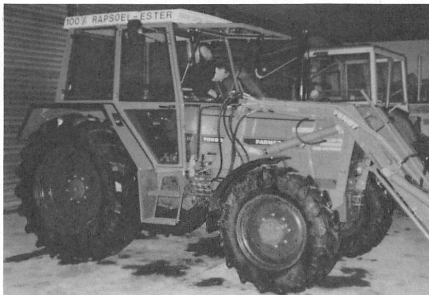
Fig 5 This tractor has been run successfully for over 400 hours on rapeseed oil ethyl esters at LAF, Braunschweig, Germany
