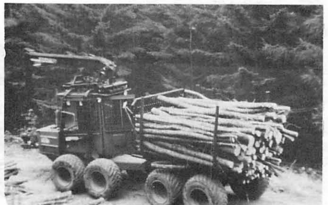
Fig 10 8 wheeled 7 tonne class 'high flotation' forwarder
