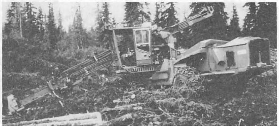
Fig 14 Sliding boom type processor
