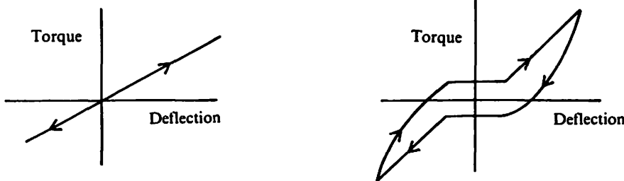
Fig 2(a) Pure spring-linear and (b) Spring with backlash and friction — non linear
