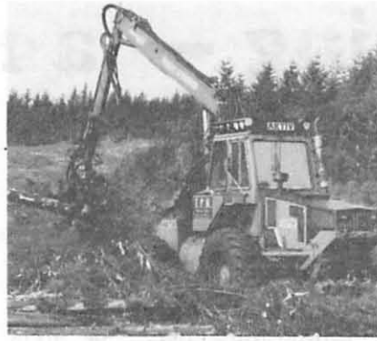
Fig 15 Grapple processor mounted on a modified forwarder chassis
