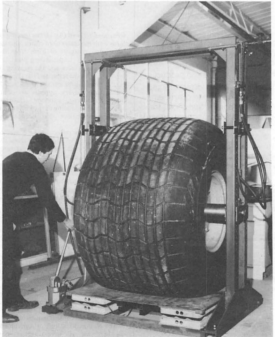
Fig 1 Tyre loading bay
