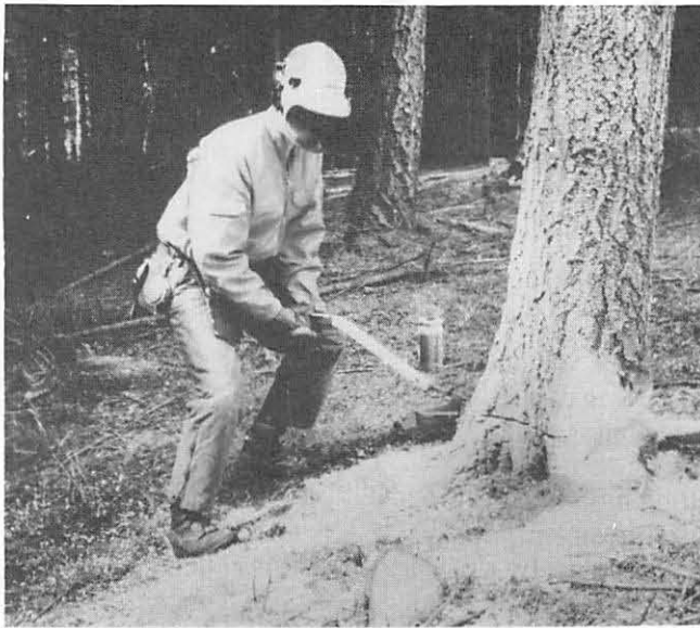
Fig 1 Felling using a conventional Breaking Bar
