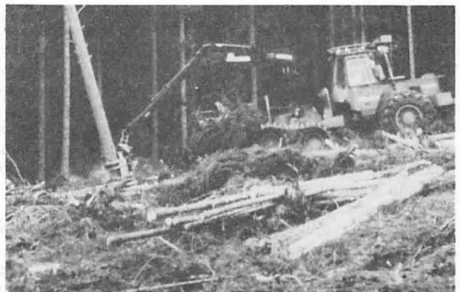
Fig 17 Harvester in operation felling a tree prior to processing
