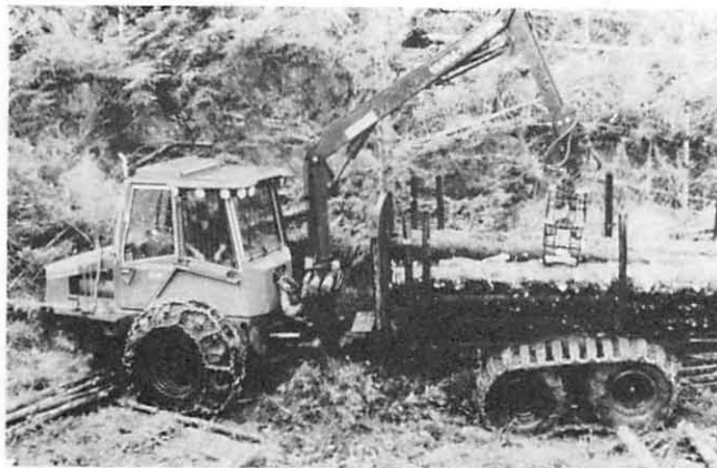
Fig 9 10 tonne class 6 wheeled forwarder fitted with front wheel chains and band tracks on rear bogie
