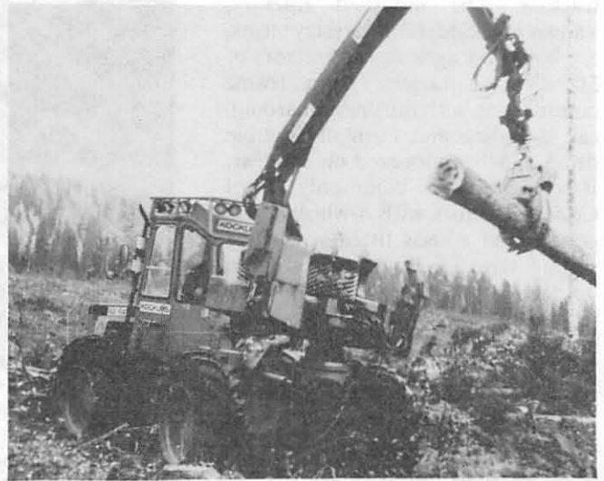
Fig 13 Compact 4 wheeled processor loading tree for processing
