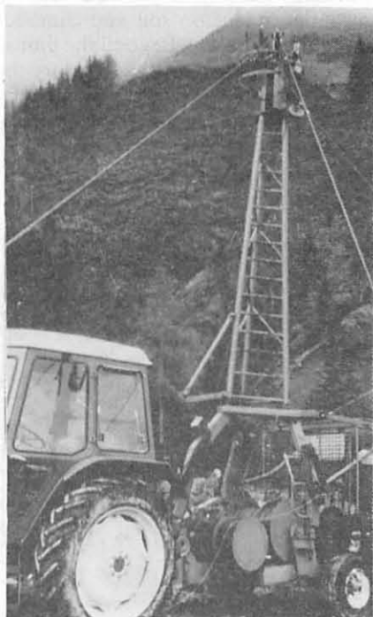
Fig 12 Trailer mounted cable crane working over a range of 600 metres
