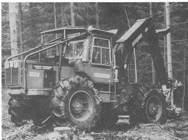
Fig 4 Purpose built Feller Buncher
