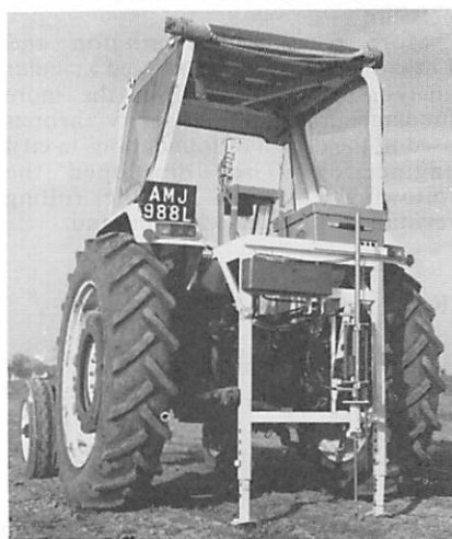
Fig 4 Tractor mounted cone penetrometer
