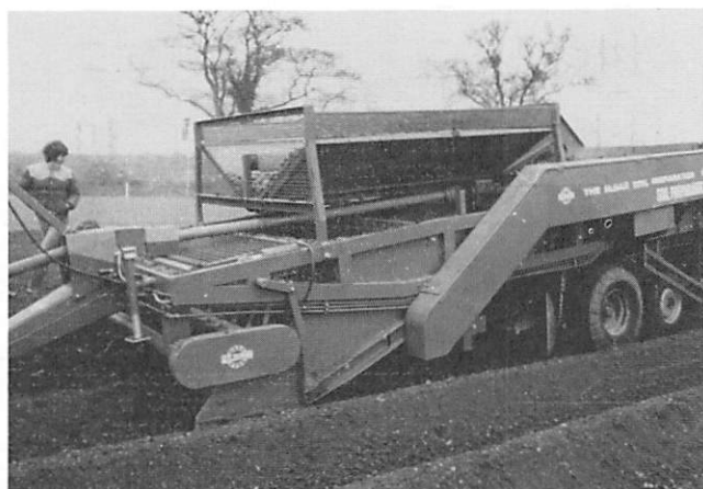
Fig 7 The Elbar multi-purpose machine equipped for (left) destoning and planting and (right) harvesting
