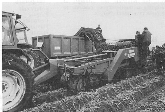
Fig 7 The Elbar multi-purpose machine equipped for (left) destoning and planting and (right) harvesting
