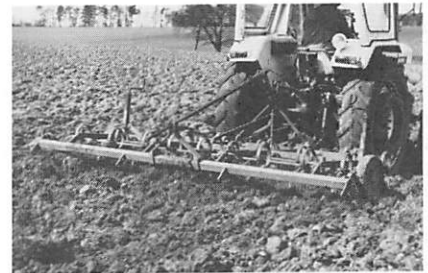
Fig 5 Triple 'K' spring tine harrow
