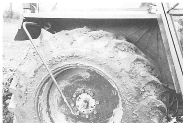
Fig 5 View of the air feed, via the support structure to the rotary valve and hence to the tyre.
