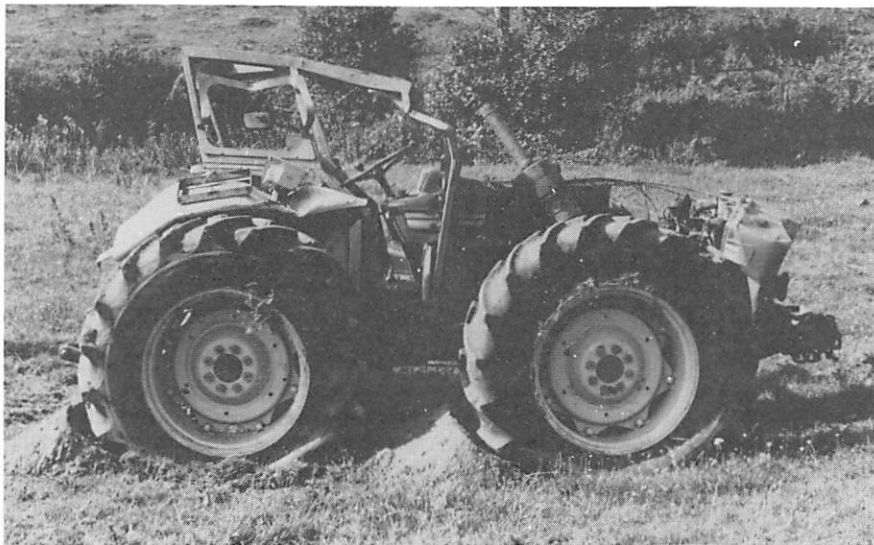
Fig 4 Extensive damage to 4-wheel drive tractor after multiple roll on very steep slope (Photograph reproduced by courtesy of the Health and Safety Executive Agricultural Inspectorate).
