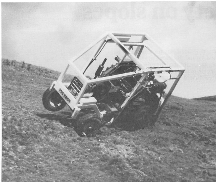
Fig 1 Radio-controlled tractor on point of overturn during full-scale experiment
