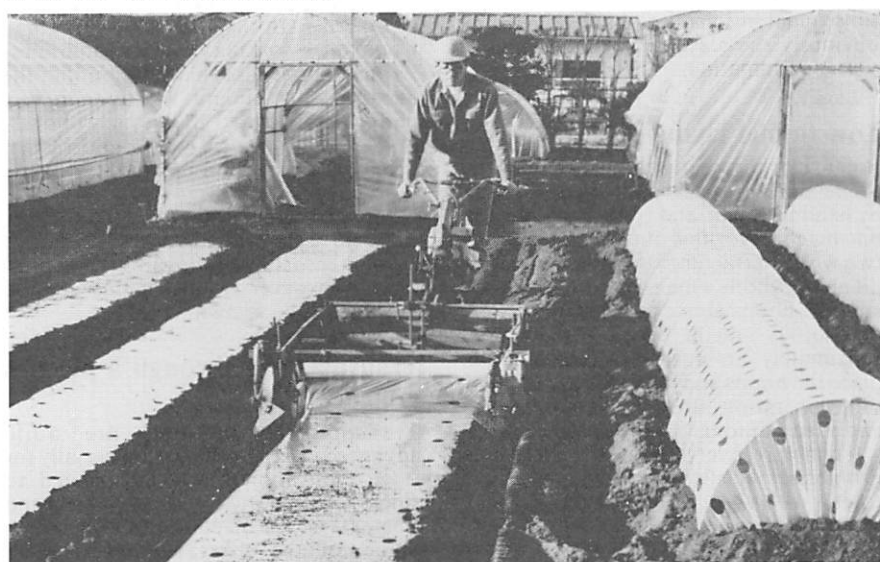
A combined ridge former and mulch layer fitted to a two wheeled tractor. Note the helical blades which throw the soil towards the centre to form the ridge
