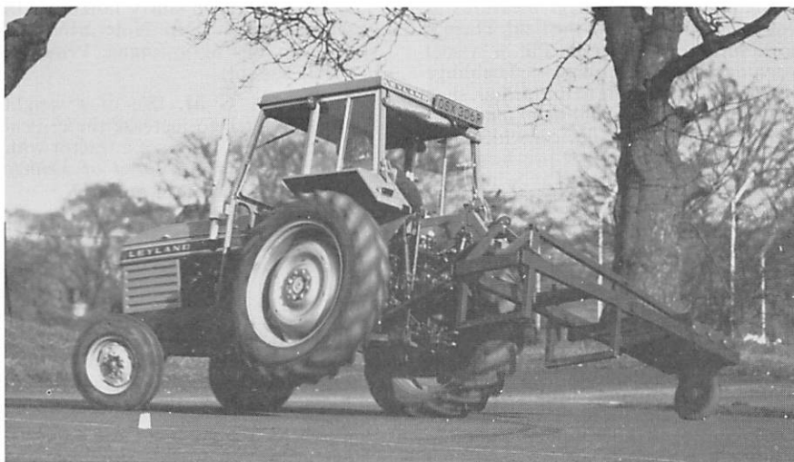
Fig 6 Tractor with outrigger to simulate the weight of a mounted rotary mower. During cornering at speed the tractor would have overturned except for the outrigger wheel
