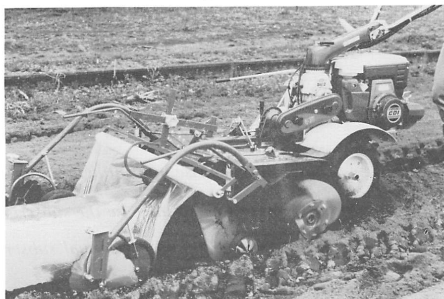
A combined ridge former and mulch layer fitted to a two wheeled tractor. Note the helical blades which throw the soil towards the centre to form the ridge
