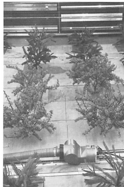
Fig 6 View of wind tunnel showing model orchard, model sprayer and air inlet section
