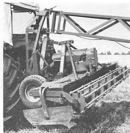
Fig 6 Space frame link connected to tractor 3-point linkage
