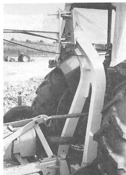
Fig 4 Two member link showing connection point to tractor drawbar
