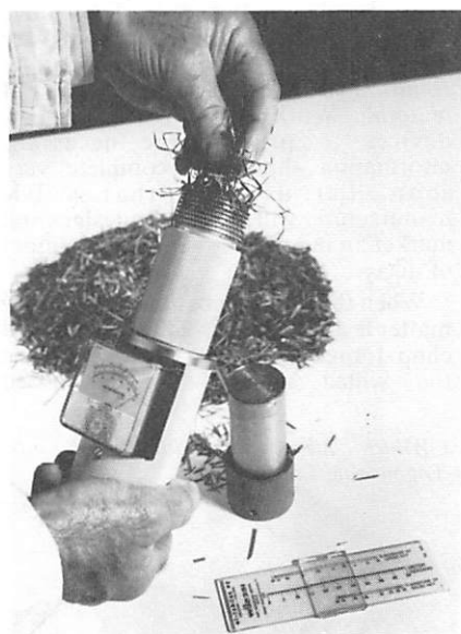
Moisture meters — (above) Froment 1210; (below left) Wile 351 meter with hay extension; (below right) Tower Silo's Cromptester Mk II (photos by courtesy of NIAE)
