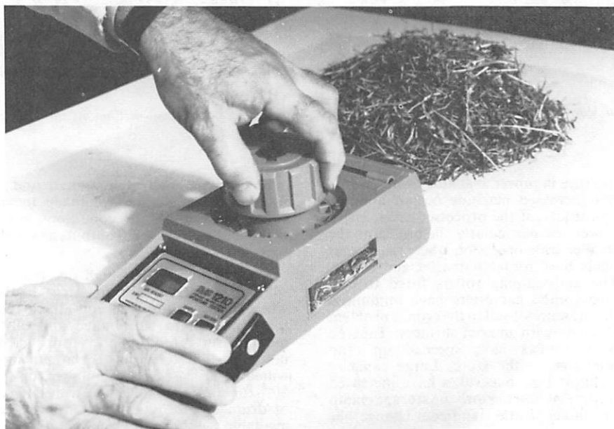
Moisture meters — (above) Froment 1210; (below left) Wile 351 meter with hay extension; (below right) Tower Silo's Cromptester Mk II (photos by courtesy of NIAE)
