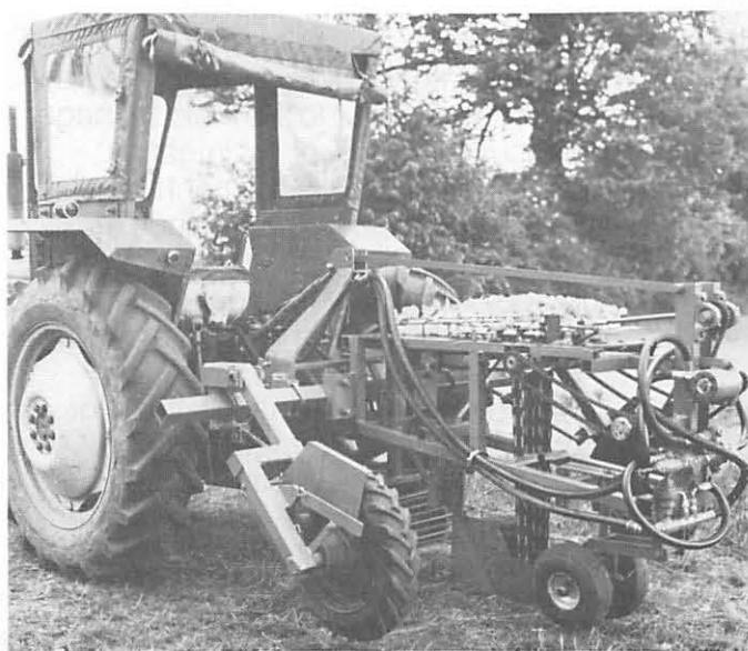
NIAE Experimental transplanter, each unit handling 5000 plants per hour. Three or four such units mounted on a tractor can be managed
