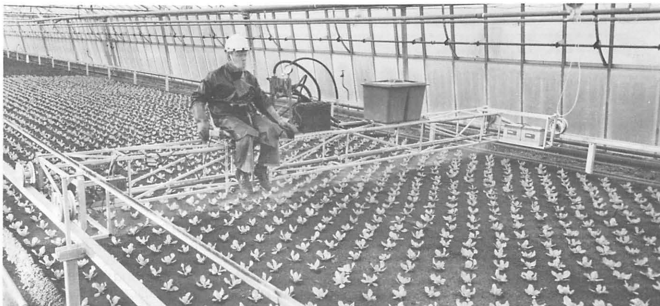
Crop – spanning gantry for glasshouse or outdoor use, obviates uneven soil compaction and need for pathways
