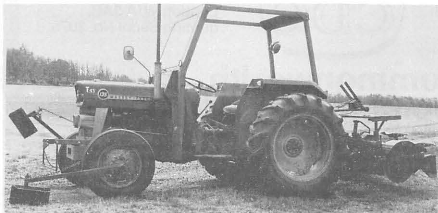
NIAE Experimental seed drill allowing accurate placement of seed and manipulation of soil environment to achieve good emergence.
