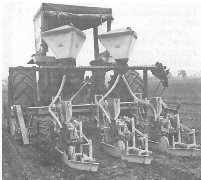
NIAE Experimental seed drill allowing accurate placement of seed and manipulation of soil environment to achieve good emergence.
