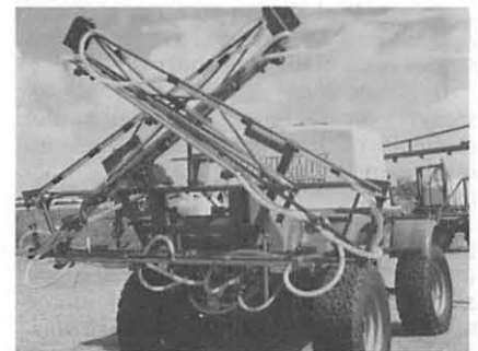
The Willmot Lightfoot-sprayer — an example of a self-propelled sprayer with vehicle suspension
