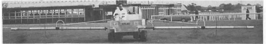
The Atlas low-ground pressure-sprayer of Cleanacres Limited with eight low pressure tyres
