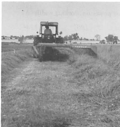
Fig 10 Immediate windrowing and coupling of windrows achieved with the machine combination shown in Fig 9
