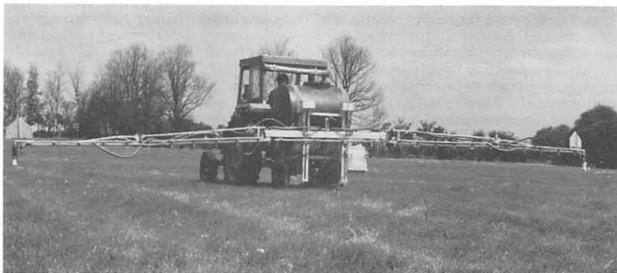
A swath matching aid - angled mirrors at the boom tips forming periscopes with a pair of mirrors on the tractor bonnet to improve the driver's view of the row of foam blobs
