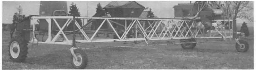
The Monotrail hydrostatically propelled gantry sprayer of Mr D Dowler which spans a 12 m swath providing good boom stability and simple and accurate swath matching
