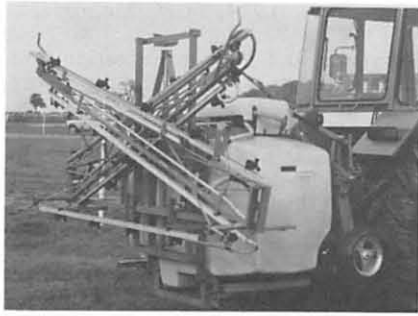
The jockey wheel picking up ground speed from the tractor rear wheel to provide automatic control of application rate with the Tecnomax AR 160 Autoregulator
