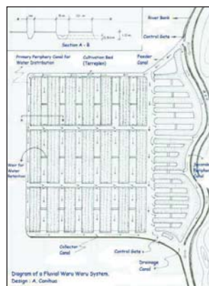
Figure 3: Plan View of a Fluvial Waru Waru designed system. (Source: Murillo, 1992)
