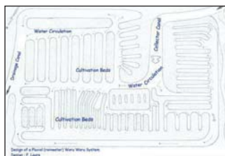
Figure 2: Plan View of a Pluvial Waru Waru designed system. (Source: Murillo, 1992) Scale guide – platform length ranges from 15m – 50 m
