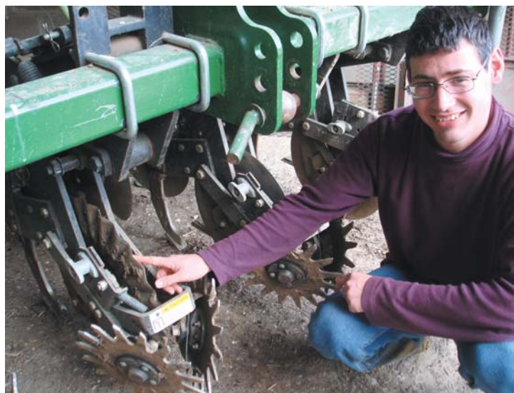
Nathan points to the star wheels for removing crop residue and fluted disc coulters for initial soil cultivation. "In the US farmers sometimes use a strip tilling machine that completes cultivation/drilling in one operation, particularly for maize on lighter soil. In the UK, particularly for sugar beet, we will more likely be looking at a machine that cultivates earlier in the year e.g. late autumn and then following with the drill in the spring when sugar beet is drilled," he said
