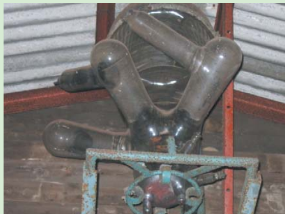
A mercury rectifier - imagination ran riot as to the design and blowing process
