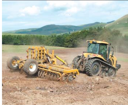
After the topsoil has been rolled down, ground preparation is completed by a six metre Knight Triple Press cultivator pulled by a 320hp Caterpillar Challenger
