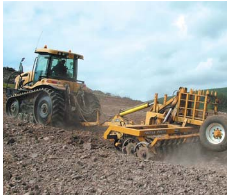
After the topsoil has been rolled down, ground preparation is completed by a six metre Knight Triple Press cultivator pulled by a 320hp Caterpillar Challenger
