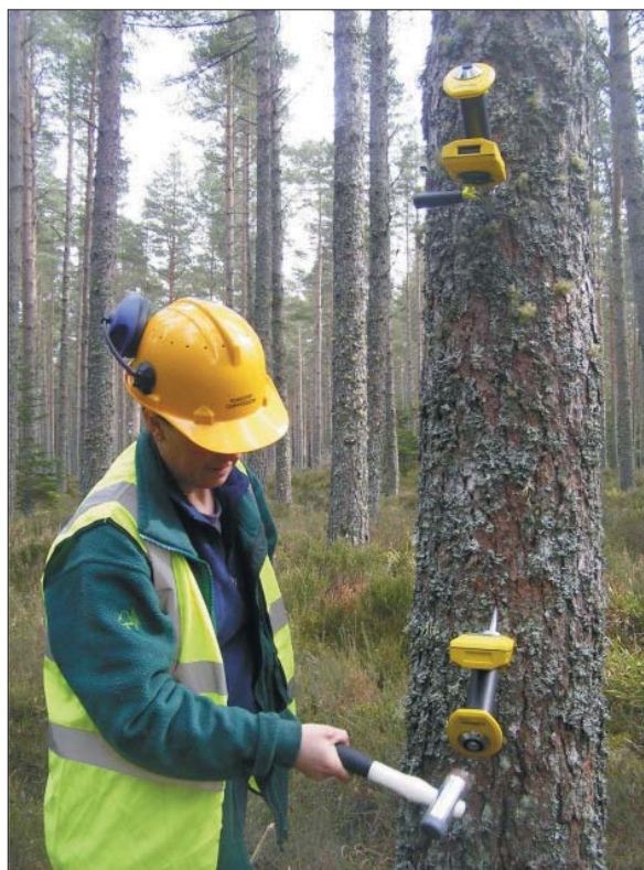
A scientist demonstrates one of the acoustic tools for assessing timber quality (photo courtesy Forestry Commission).
