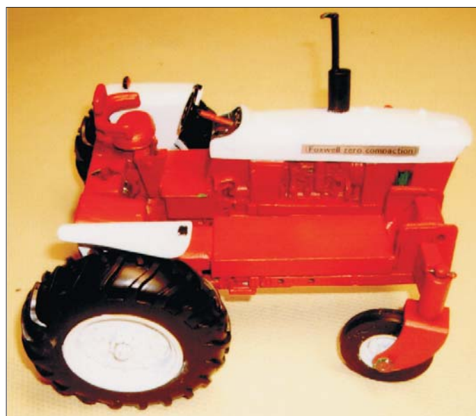
Fig. 6 After removing the cross beams and torque arm, the control unit and slave drive unit can be connected together to provide a shipping configuration for the 'gantry' tractor
