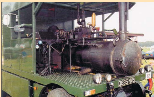
Spider MK2 steam powered vehicle designed and built by John Kilgour. The vehicle requires coal or wood as its fuel and will generally carry 1.2 tons of water and 1.5 tons of coal. The boiler is based on a 3:4 scale Foden working at 225 psi and delivers sufficient power to propel the vehicle, based on modified Bedford RL chassis, at a cruising speed of 25 mph
