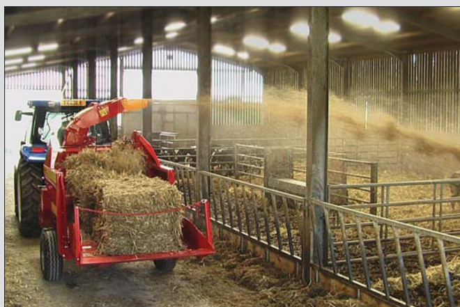
The Tomahawk 8080 dual chop can chop straw long (pictured) for loose housing or short for open cubicles, poultry, etc., at the flick of a switch
