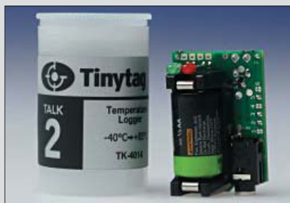
Tinytag Talk 2: improved version of Gemini's impressive range of temperature, humidity and voltage data loggers
