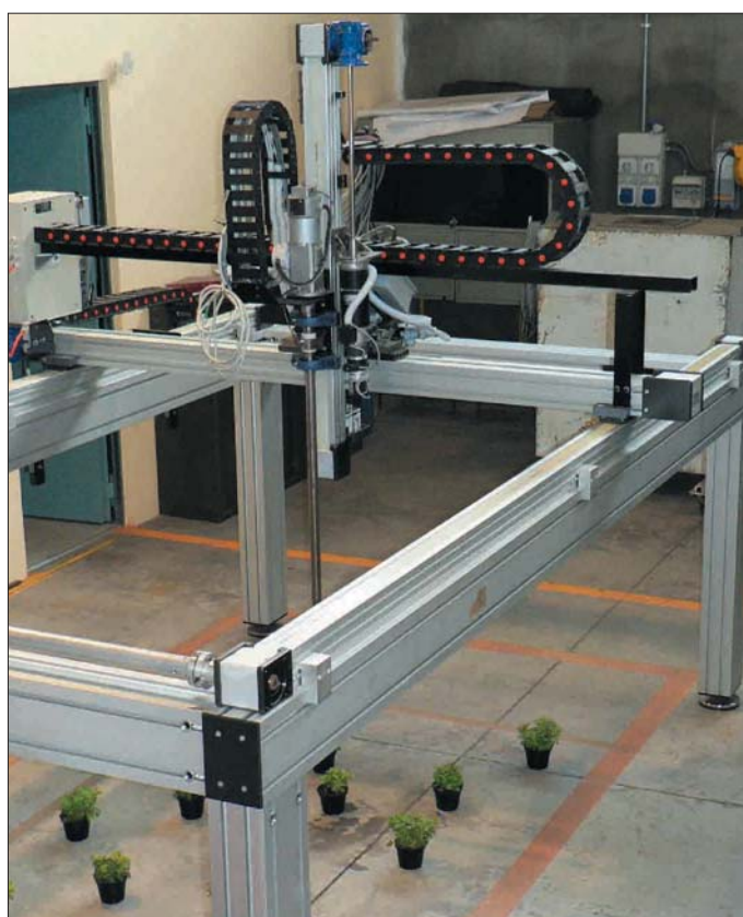
Fig. 2 The second prototype has a Cartesian structure; this allowed to improve performances and operations accuracy
