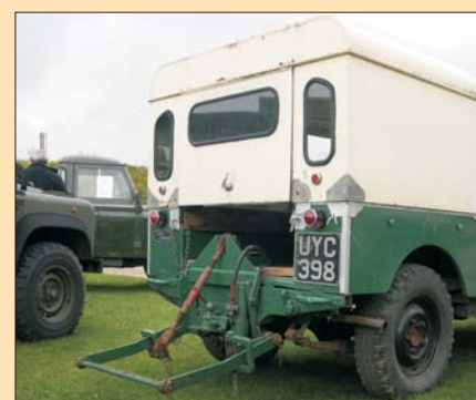
The same vehicle with a rear mounted 3 point linkage displayed on the Dunsfold Collection stand at the Land Rover Marque event, Heritage Motor Centre, Gaydon, in May 2006 (see http://www.heritage-motor-centre.co.uk/ ) [Photo: Stuart Martin]
