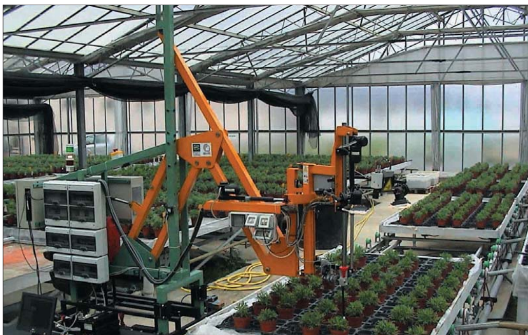
Fig. 1 The first prototype was designed to operate in a fixed position along a belt-conveyor displacement system. Its mechanical structure leads to a small encumber
