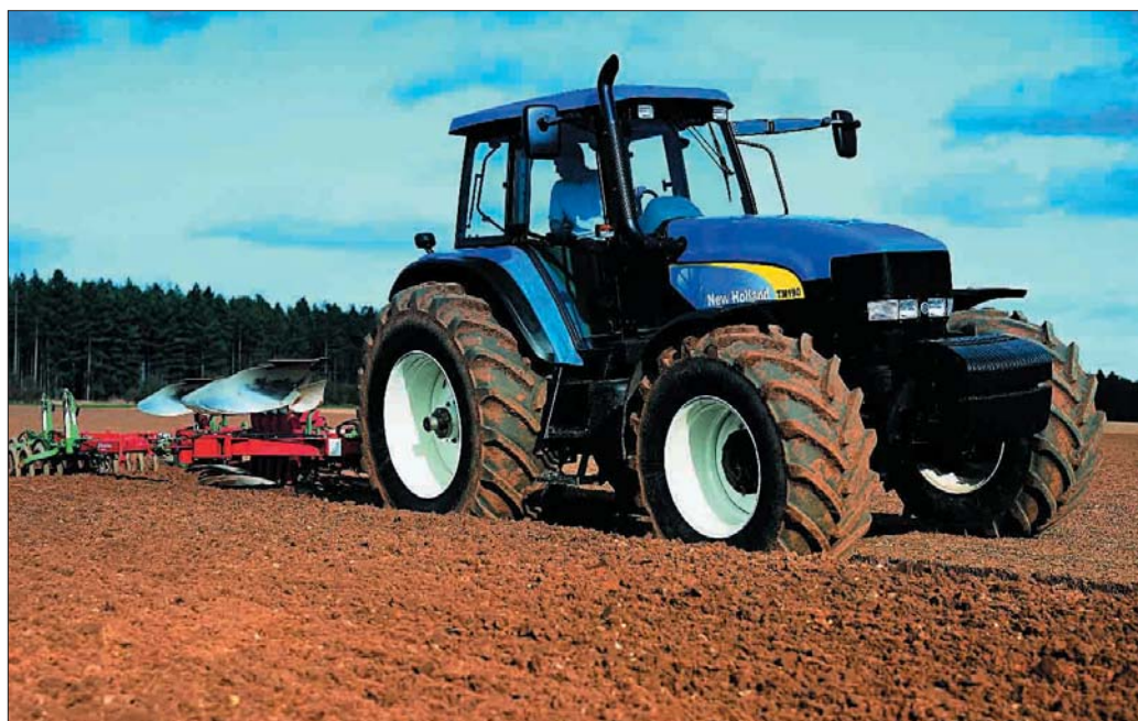
New Holland worked a standard 146 kW TM190 tractor non-stop for 500 hours using 100% biodiesel, to reproduce the work patterns of its most intensive-working customers, such as large-scale farmers and contractors
