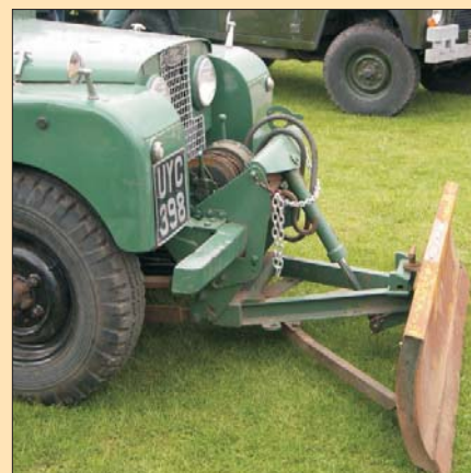
A 1955 86 inch wheelbase Land Rover Series I with a front mounted straight snow plough blade made by Howie [Photo: Stuart Martin]
