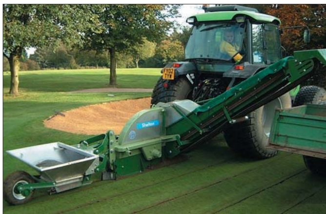
Single leg gravel band drainer working on golf green after hollow coring
