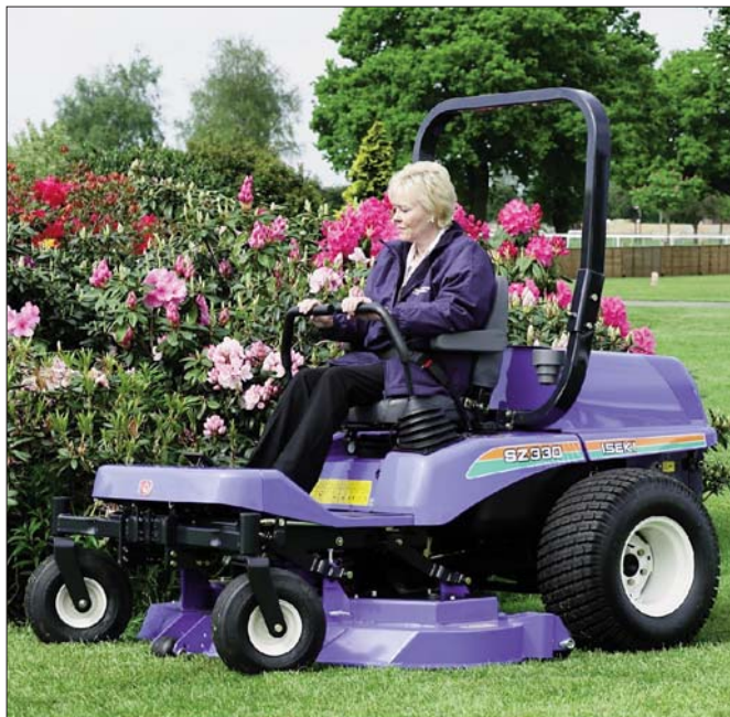
Iseki SZ330 features a floating rear axle which aids the contour mapping when mowing
