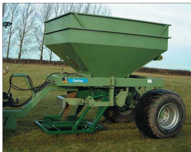
Shelton 6-tonne Fastflow gravel and sand hopper placing gravel in trench.
