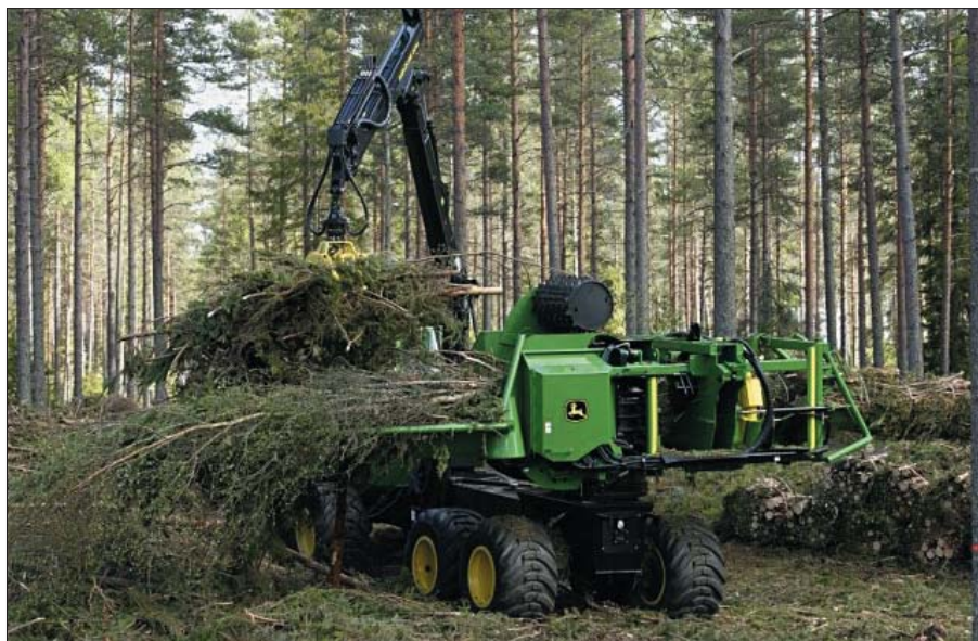
John Deere's 1490D slash bundler; the bundling process in addition to other functions of the machine are controlled via the Total Machine Control system®
