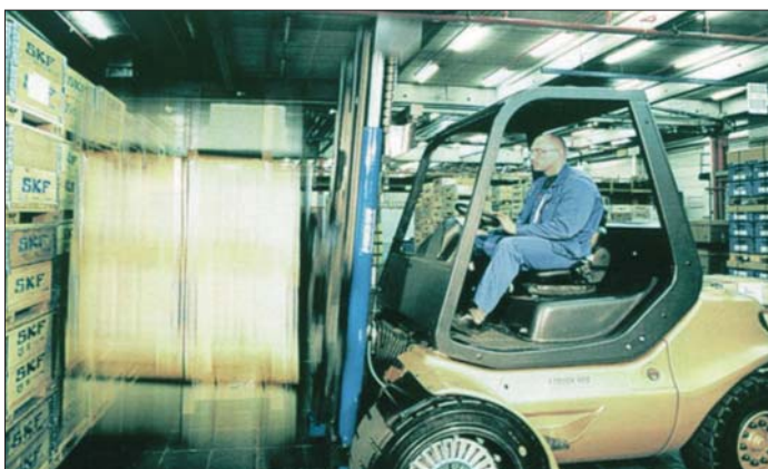
Fig. 2 The fully electric SKF forklift truck demonstrates the high performance of electric linear actuators as an alternative to hydraulics
