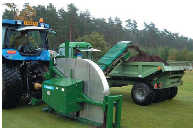
Supertrencher laying pipe on a golf fairway; a 4-wheels in line dump trailer removes soil from the conveyor ring
