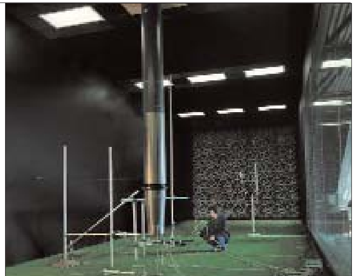
Atmospheric Flow Laboratory, with preparatory work for an experiment to simulate thunderstorm downbursts which produce short-term, extreme, surface winds
