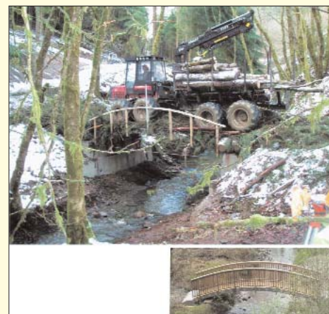
Arduous prototype testing with 36 t forwarder meets safety requirements for the next generation of heavier hikers traversing the conversion to provide an attractive footbridge (bottom)!
