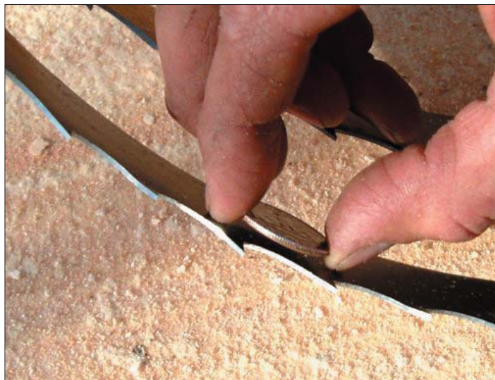
Very thin kerf means less sawdust and more timber
