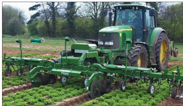
Garford built Robocrop hoe, running Tillett and Hague Technology Ltd's vision guidance and tracking software and operated by Intercrop (a large salad producer) in Kent. Three cameras are used to track and hoe three separately planted beds in one pass.
