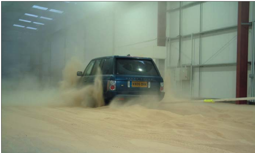
Fig.6 Controlled evaluation of a Range Rover in simulated desert sand conditions
