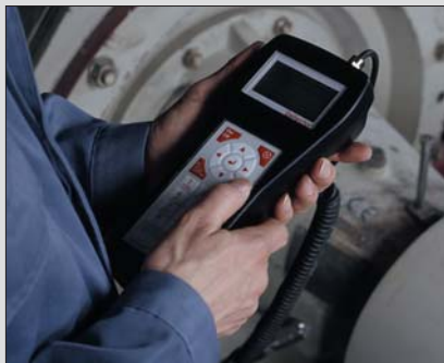
Schaeffler (UK)'s Detector III is the latest damage diagnosis instrument from FAG Industrial Services
