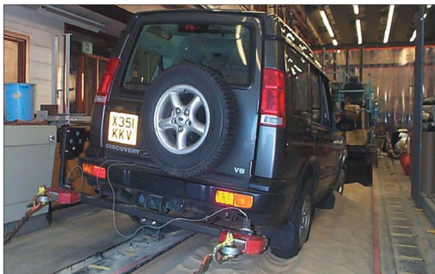
Fig.1 Traction control system evaluation for the Land Rover Discovery in the existing 1.75 m wide x 20 m long soil bin (in desert sand)
