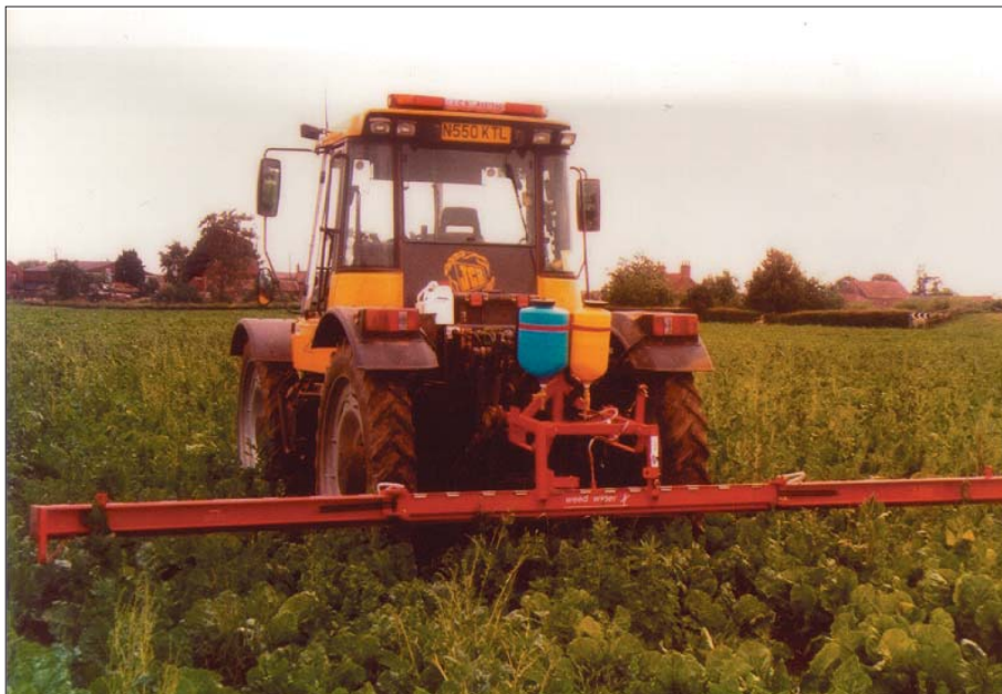
The WeedSwiper from Micron Sprayers - eliminates weeds without making any contact with the crop
