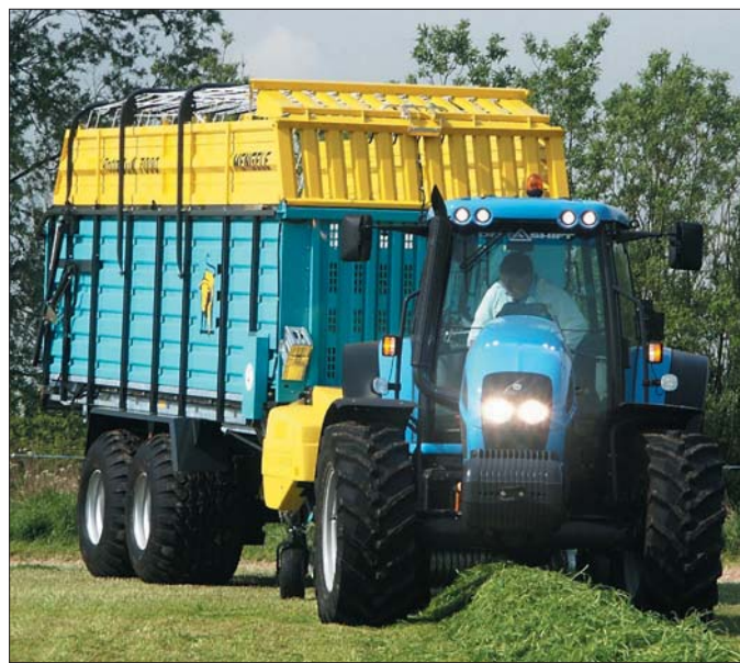
A 58 m 3 capacity model from Mengele's Rotobull extended range of self-loading forage wagons
