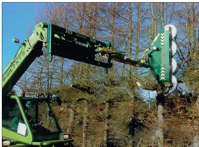
The LRS2001 and LRS2401 Quadshaw models from Spearhead have respective cutting capacities of 15 and 20 cm and cutting widths of 2 and 2.4 m
