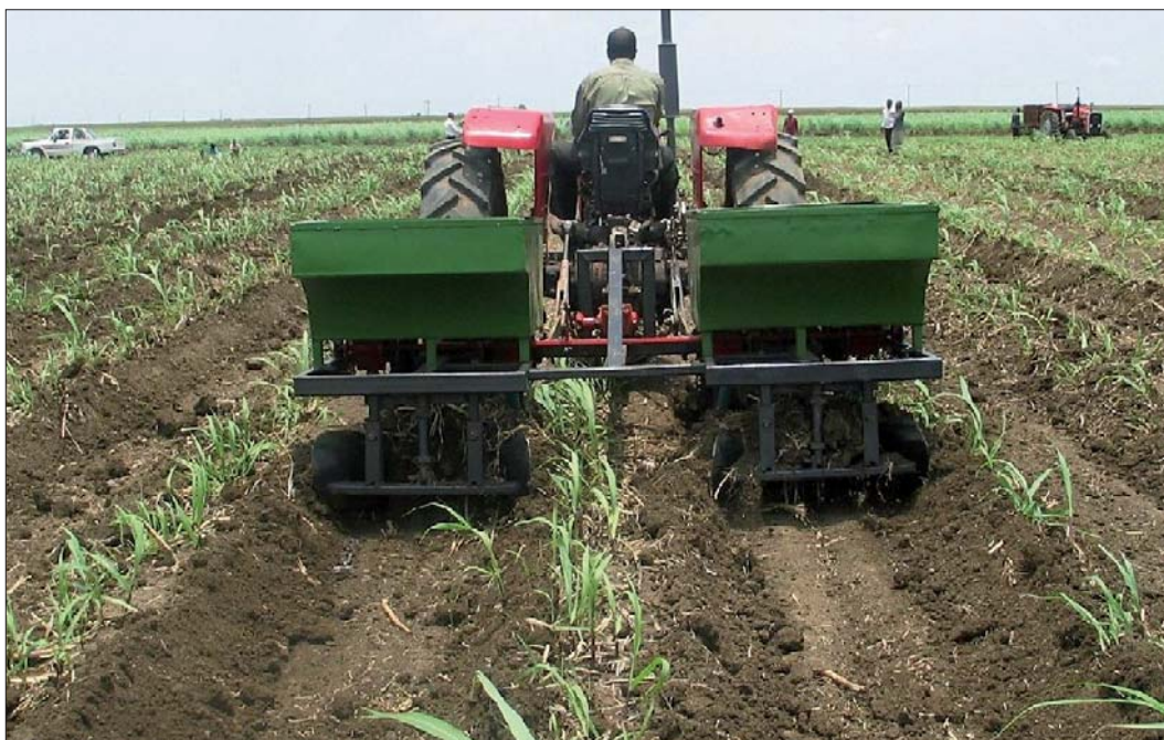
The cane field cultivator; a two-furrow, tractor mounted machine designed to comprise functional components of a chisel cultivator, two fertiliser applicators and a ridger.
