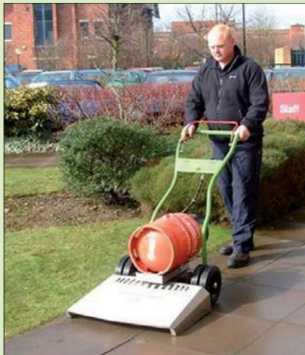
Calor LPG powered pedestrian weed burners are an effective solution to weed control for those seeking an alternative to herbicides
