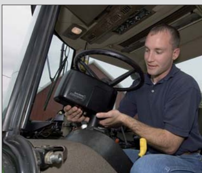
Universal AutoTrac - John Deere's first aftermarket automatic guidance system for tractors and self-propelled equipment
