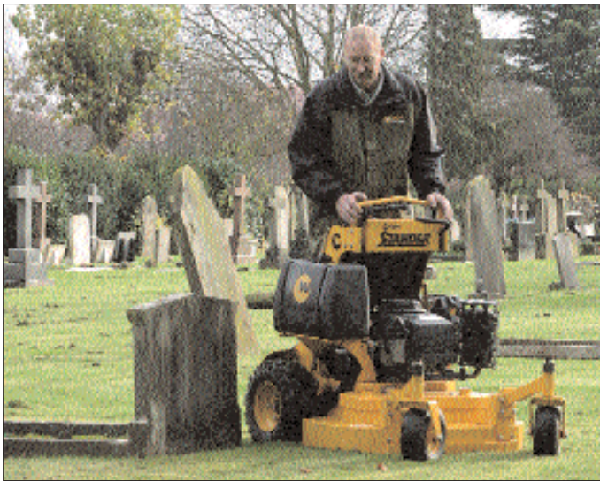
Stander range have integral operator platforms, eliminating the fatigue of pedestrian mowing
