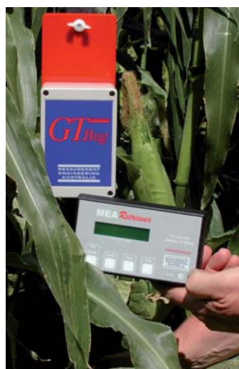
The G-Bug – a small battery powered data logger connected to sensors and buried at various soil depths monitors soil moisture content
