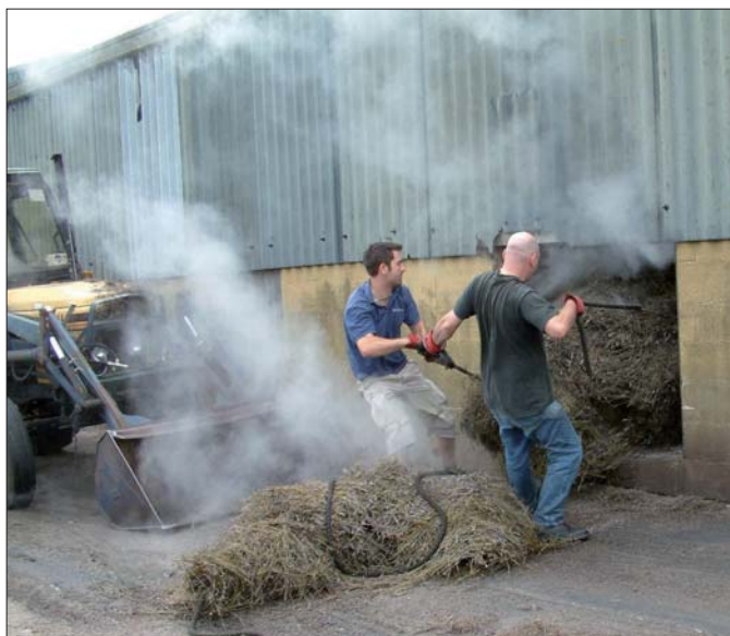
Ropes are used to extract the near sterile dross from a still once the distillation cycle is complete
