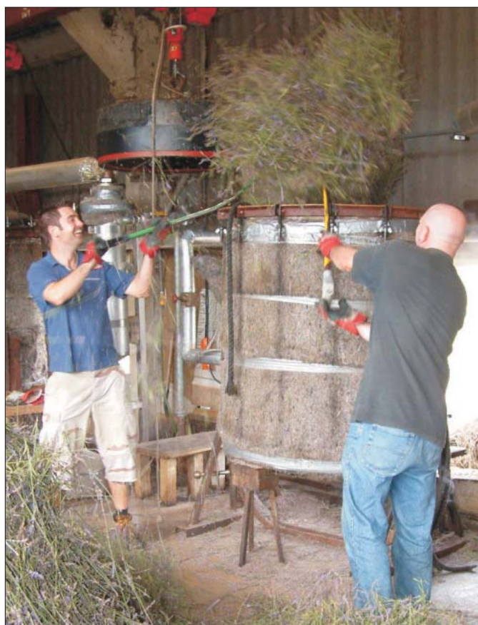
Distillation of lavender oil continues to use pre war copper stills into which the lavender is forked manually
