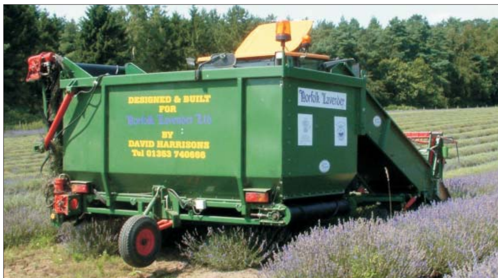
The hopper is an adaptation to the original cutter, where the lavender piles up in a hopper which is now situated directly behind the tractor
