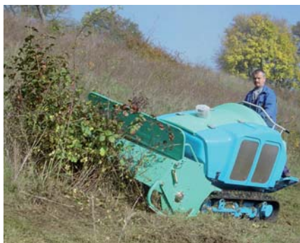
The Kyoisha hammer knife mower has a very low center of gravity; the static roll over angle is 60° to the side and 70° to the front and rear side enabling it to work on steep embankments.
