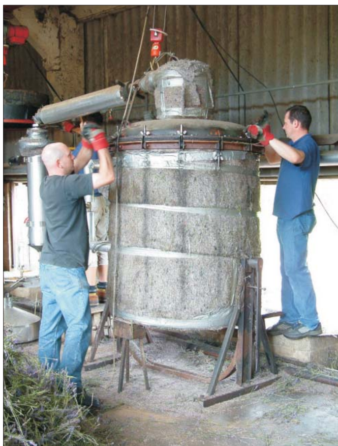
The still lid is clamped down and processed for twenty minutes at a pressure of between 3.5 and 5 bar
