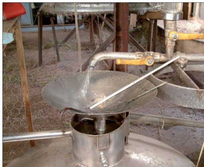
Separator: the vessel in which the lavender oil and water settle until the oil separates and sits on top of the water, ready to be tapped off
