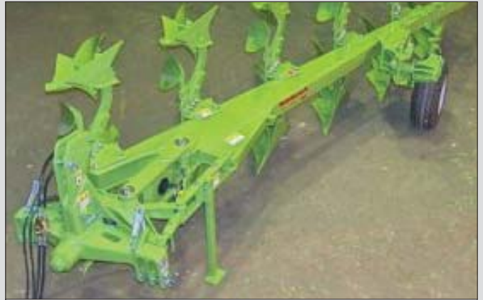
A six furrow Dowdeswell 110 series plough with shearbolt protection
