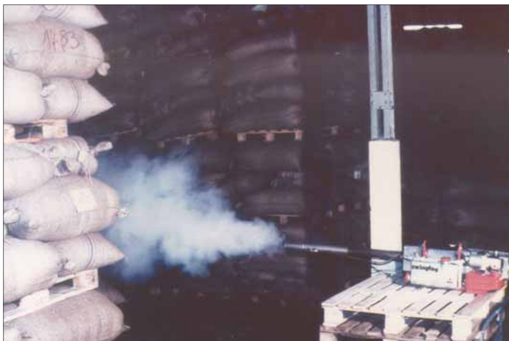
A swingfog thermal (hot) fogger from Allman, operating in a food storage area
