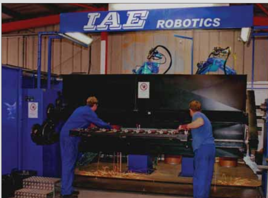
The Motoman twin-robot welding cell in action at Industrial and Agricultural Engineers (IAE)
