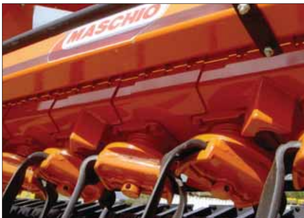
Maschio's DM Rapido Plus from RECO has additional protection on the underside circular blade holders and stone deflectors between the alternate rotors
