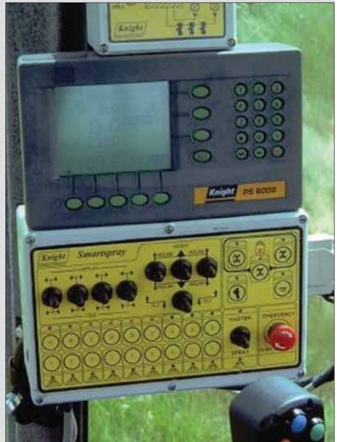
Knight's full fingertip control system (FCS) has two control panels and a joystick, all interlinked to provide full logic
