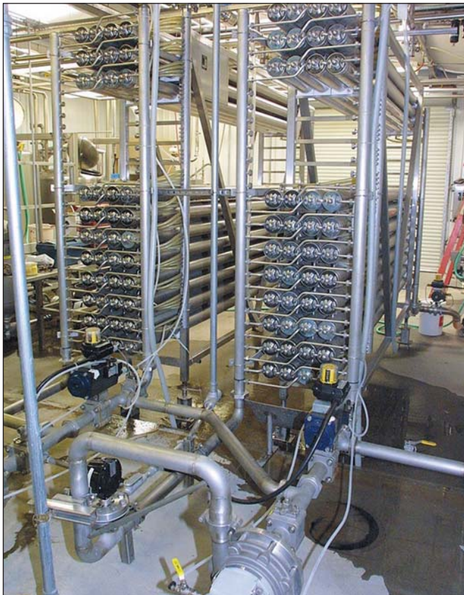
The membrane filtration plant, installed at National Raisin Company, incorporates 80 Model B1 filtration modules and is designed so that it can easily be expanded 50 percent to 120 modules to meet increased demand in the future.
