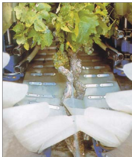
Efficient picking by horizontal shaking rods into redesigned baskets which improve the sealing between the vines
