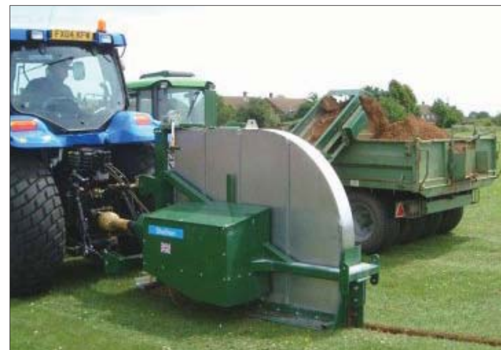
Shelton Supertrencher, and Shelton 4-wheels-in-line High Lift Trailer draining a sports field with superb clean surface finish
