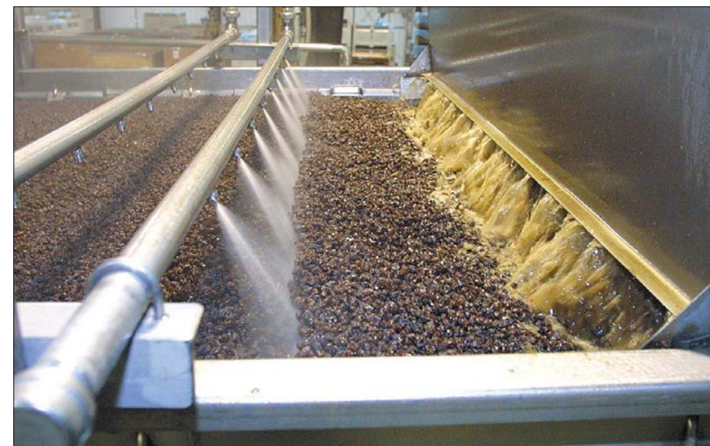
Raisins at National Raisin Company enter the washing system by conveyor, at a rate of 200 tonnes per day.
