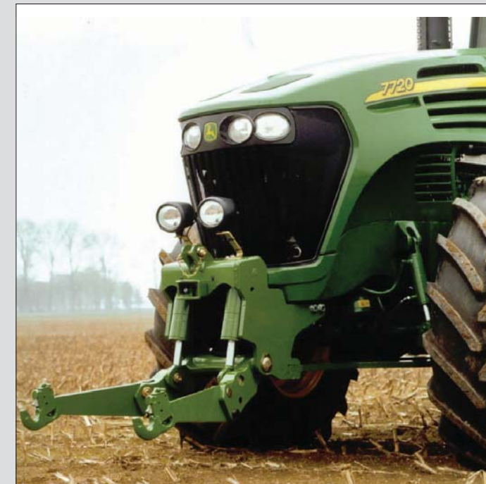
Lynx Engineering's new 5 t Frontline linkage system attached to a 7720 John Deere tractor from its new 7020 tractor range
