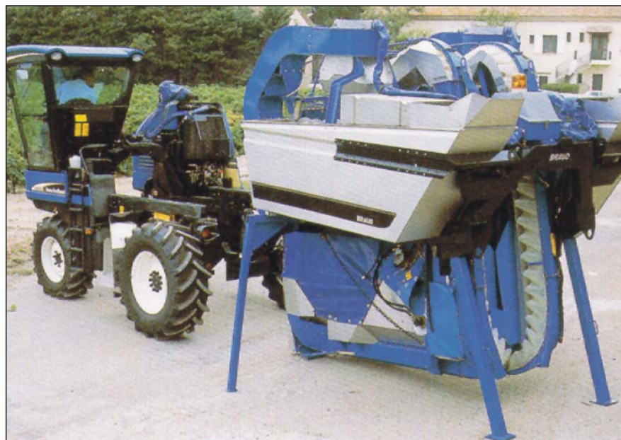
Fast detachment of the harvesting unit
