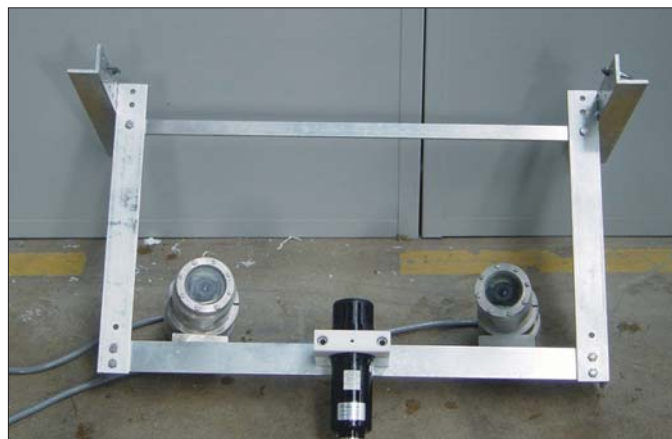
Fig. 1 The acousto-optical sensor developed for this project; stereo-camera pair with the Tritech sector-scan sonar in the middle
