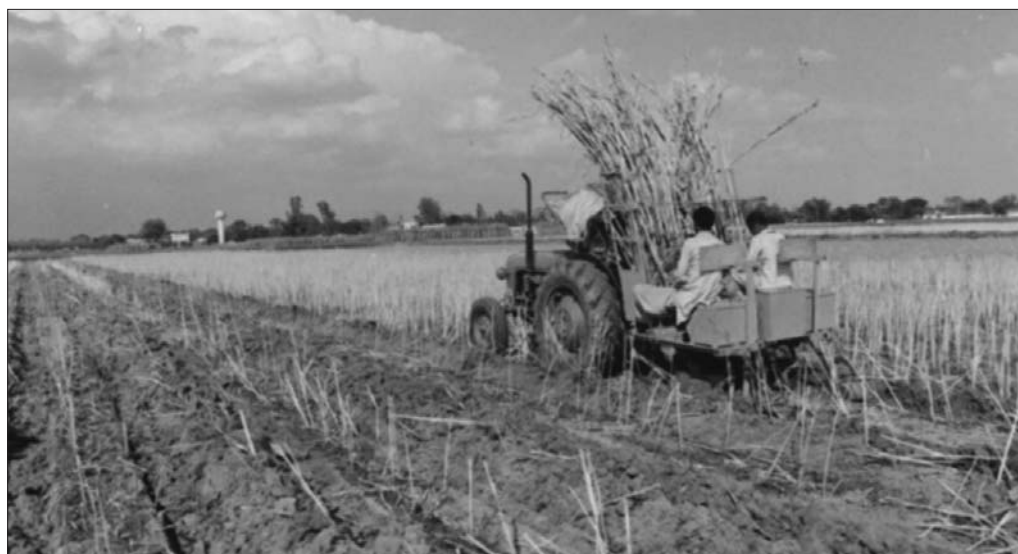
Ground wheel driven cutter-planter, in action, planting in a mustard field
