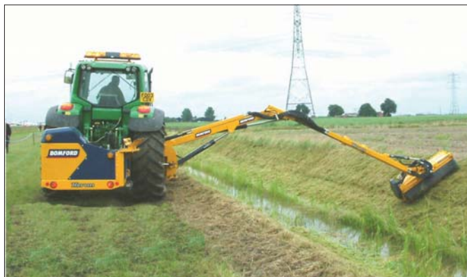
New long reach flail cutter designed to meet increased requirements for waterways' maintenance, embankments and other uses involving a reach of up to 9.2 m
