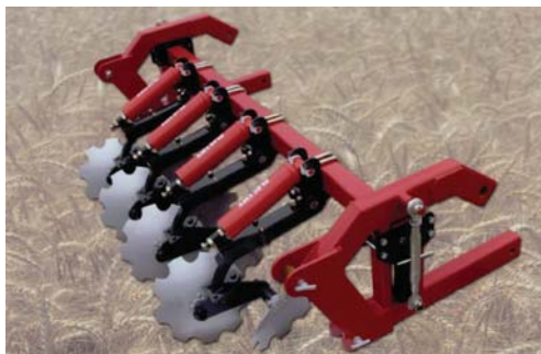
New toolbar option, using four pairs of angled discs fitted to same spring loaded tine as existing toolbar; cuttaway discs for greater cutting, mixing and inversion action in heavier conditions
