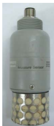
Prototype patented dielectric tensiometer, currently undergoing field trials.
