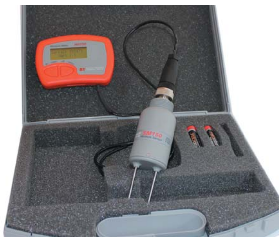
SM150 kit - one of a range of soil moisture kits available that are robust, easy to use and accurate. These sensors can also be buried and attached to data loggers for continuous monitoring of subsurface water changes.
