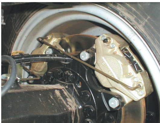
Twin caliper brake installation with cable to ABS sensor
