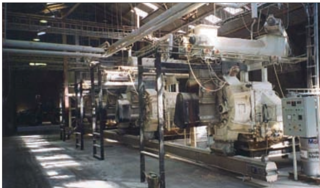
Pelleting machines, three visible, each producing pellets for consumption by wood pellet boilers or stoves (Photo: British Biogen - www.britishbiogen.co.uk )
