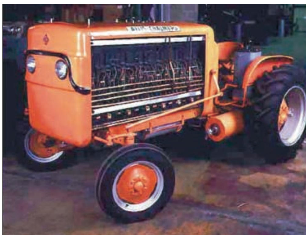
Fig. 3 Allis Chalmers fuel cell powered tractor, 1959 (Courtesy: Smithsonian Institute)
